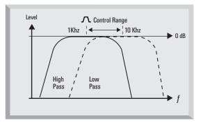
control is adjusted, both filters change in unison, blocking the high and low signals so that only a narrow band of frequencies can pass between them.
