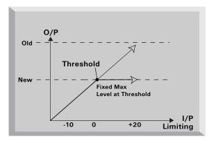
• A compressor reduces changes in volume, so that the dynamic range of the compressed signal is lower than the dynamic range of the input signal
