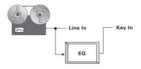
Now, you can use the key input to control the compression of the original signal. The original signal is compressed as if the dominant instrument had been attenuated.
