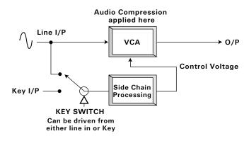
key input. Note that the key input signal is not output from the unit, it is the original input that is compressed, but compression is applied as if the key input signal were being compressed.
