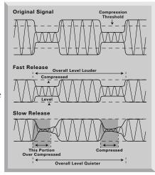
release time for the whole input signal; instead, you can use the Auto button. Auto reacts to the dynamic range of the input, so the higher the signal is above the threshold, the longer the release. This means that fast signals that aren't compressed hard have a fast release time, while longer signals release more slowly, which makes the compression in context with the signal.
