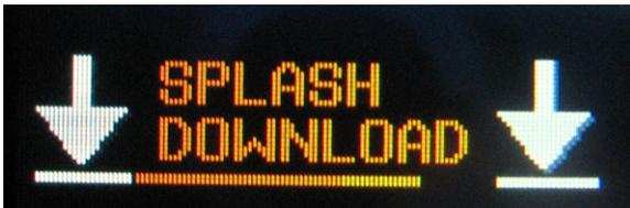
Once the keypanel is finished processing the download, the keypanel begins to reprogram. The keypanel flashes a Reprogramming: Do Not Turn Off icon in the display panel. This can take several minutes.
