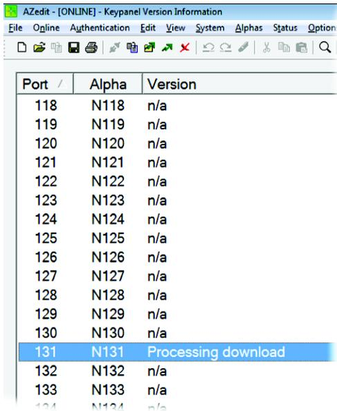
13. Verify the keypanel displays the **Processing Download icon with progression bar**.
