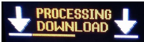
Once the keypanel is finished processing the download, the keypanel begins to reprogram. The keypanel flashes a Reprogramming: Do Not Turn Off icon in the display panel. This can take several minutes.
