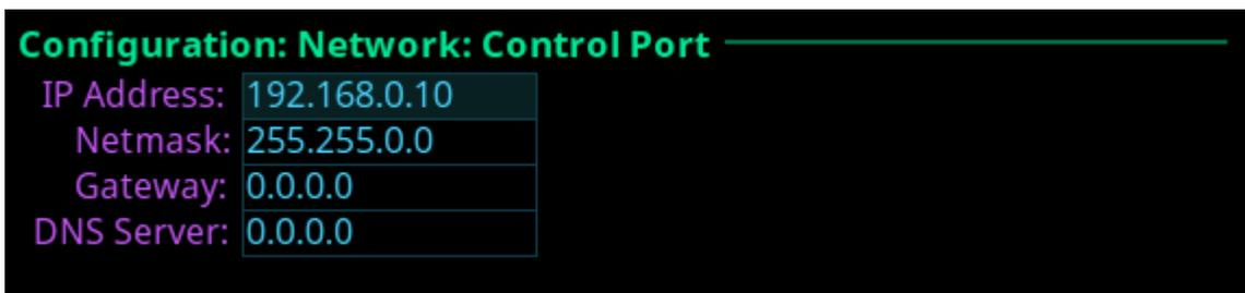
FIGURE 53. Configuration | Network | Control Port
