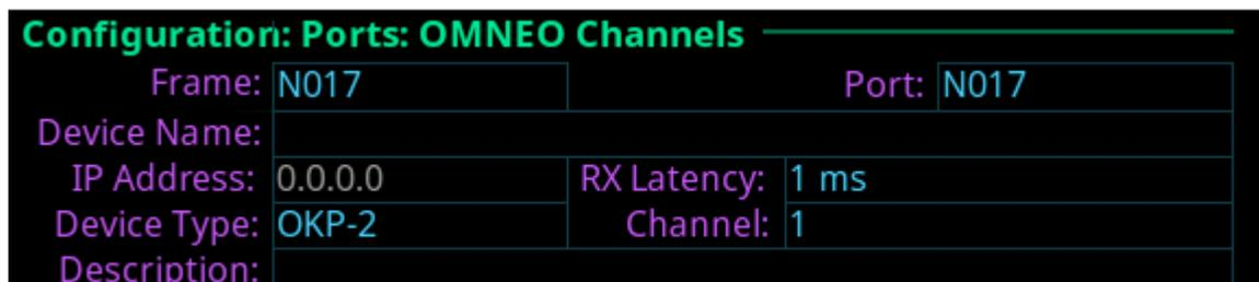
**IMPORTANT:** If the intercom system contains only one ODIN frame, the Frame field is not displayed. If the intercom system contains multiple ODIN frames, the Frame field activates allows ports in other frames to be selected and configured. While the Frame field is highlighted, press the **right encoder knob** to activate the field. Once activated, turn the right encoder knob to select another frame in the system.
