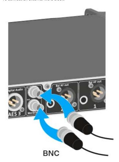
$\, \triangleright \,$  Use a coaxial BNC cable (75  $\, \Omega )$  to connect the external word clock to the Wordclock In input.
