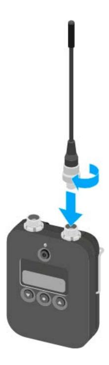
The antenna can be connected to the antenna socket very easily in only one direction. Do not use force to connect the antenna to the bodypack transmitter antenna socket.
