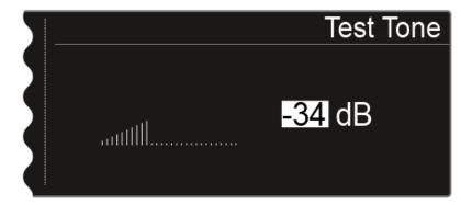
While the test tone is played back, the transmitter audio signal is muted.
