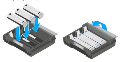
To insert the B 61 battery compartment into the SK 6000 bodypack transmitter:
