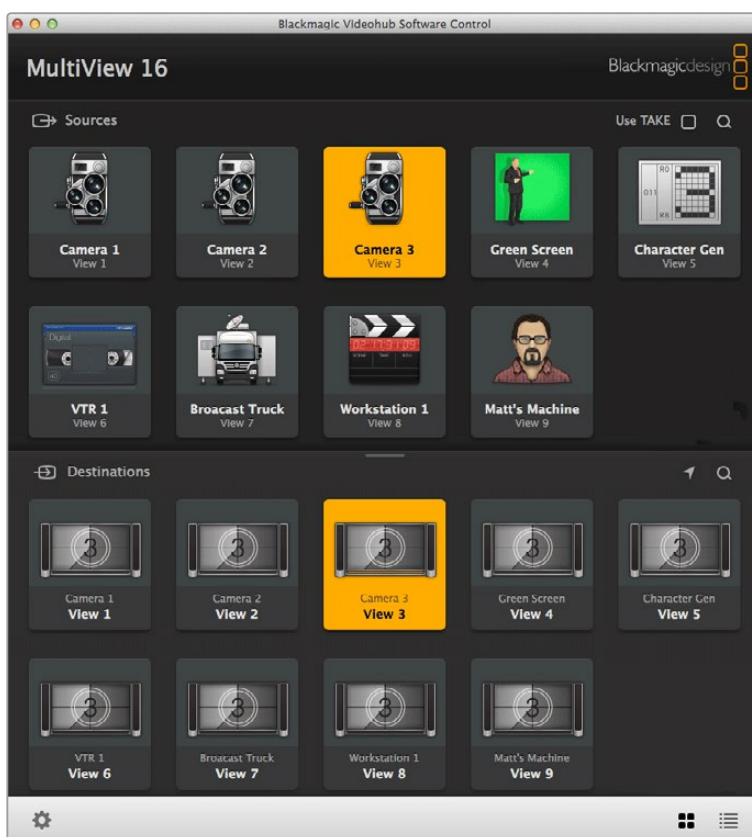
You can use Blackmagic Videohub Control to route Blackmagic MultiView 16's sources to different views
