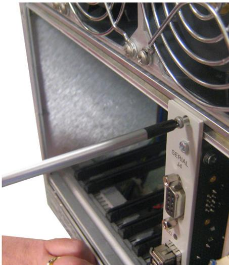
5. Using the supplied screws, tighten the **OMI back card to the frame**.
