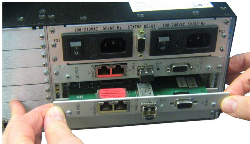
4. Ensure the **OMI back card is seated properly against the OMI front card** and is sitting firmly in the frame.
