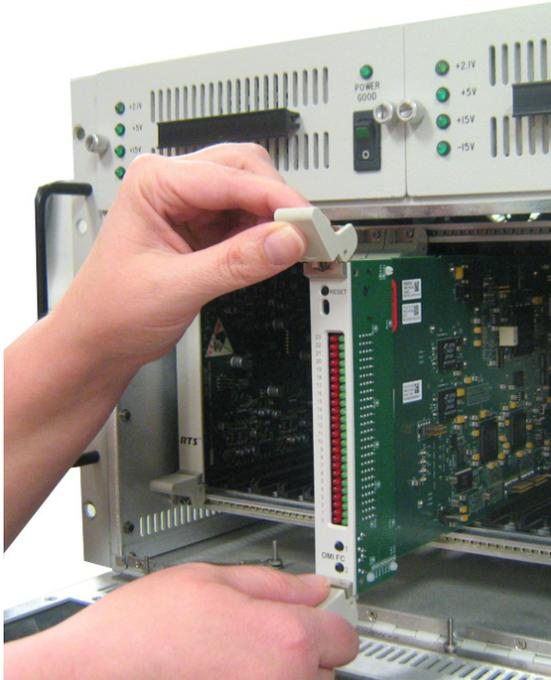
3. On the back of the ADAM frame, carefully insert the **OMI back card**, aligning it with the OMI front card.
