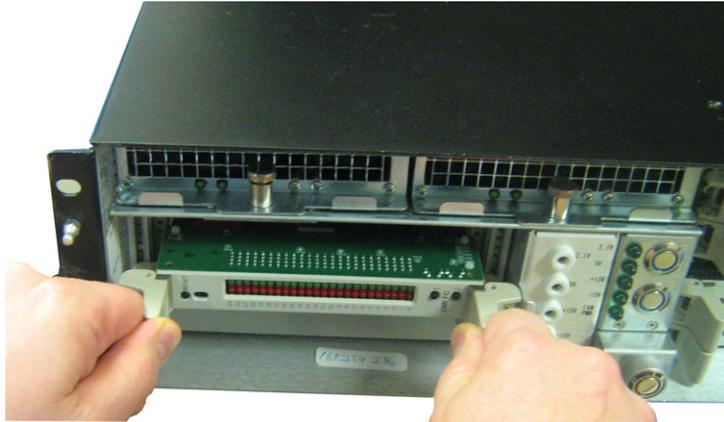
2. Using the card ejectors, tighten down the **front card** by pushing it into the slot.
