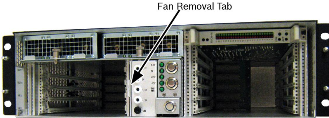
4. Using the fan removal tab, pull the **fan unit** from the ADAM-M chassis.
