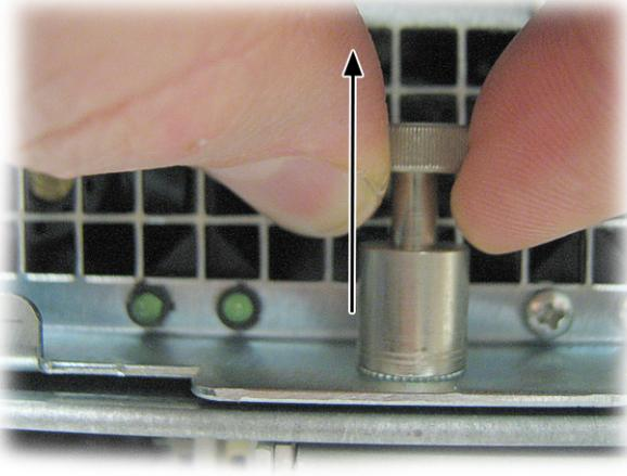
3. Rotating counterclockwise, rotate the **finger lock** half a turn.
