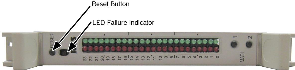
**FIGURE 5.** Reset Button and LED Failure Indicator
