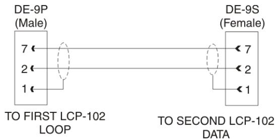
**FIGURE 11.** Cable to interconnect two (2) LCPs.
