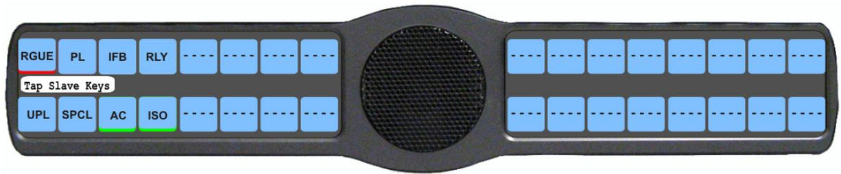
9. Tap **down** on the keypad keys you want to be activated when the master key is selected.
