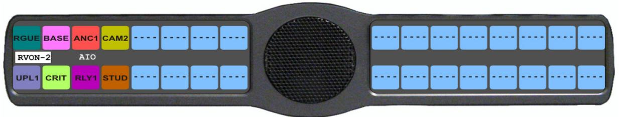
**NOTE:** If an RVON-I/O is connected to the keypad, RVON-I/O replaces the AIO menu option.
