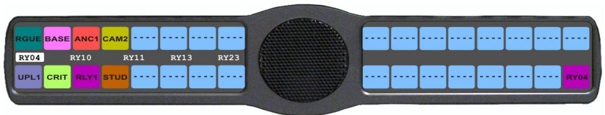
6. Using the 3(↑) or 6(↓), select the **relay** you want to assign to the keypanel key.
