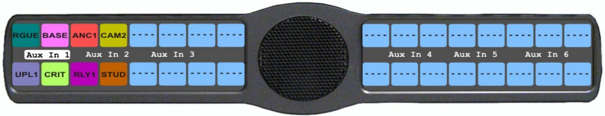
8. Using the 3(↑) or 6(↓), select **Aux In 1**, **Aux In 2**, **Aux In 3**, **Aux In 4**, **Aux In 5**, **Aux In 6**, **Front Hdst**, **Front Mic**, **Matrix In**, **Rear Hdst**, **Rear Mic**, **RVON Ch1**, or **RVON Ch2**.
