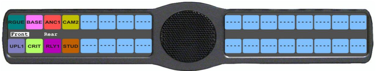
**NOTE:** All four (4) mics cannot be enabled at the same time. If three (3) mic sources are turned on, the rear panel mic is not available. For example, if the front panel mic, the front headset mic, and the rear headset mic are *Enabled*, the rear panel mic is not available.
