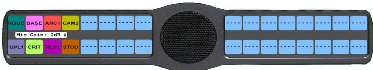
10. Using the 3(↑) or 6(↓), scroll to the **mic gain level** (in dB) you want.
