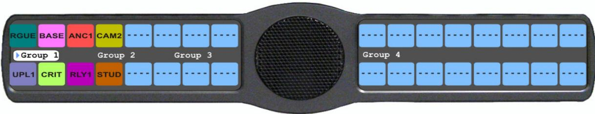
12. Using the 3(↑) or 6(↓), select the **group** you want to assign the GPIO Input to.
