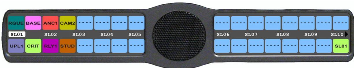
6. Using the 3(↑) or 6(↓), select the **Special List** you want to assign to the keypad key.
