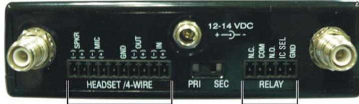
Base Station rear panel showing HEADSET/4-WIRE and RELAY connectors
