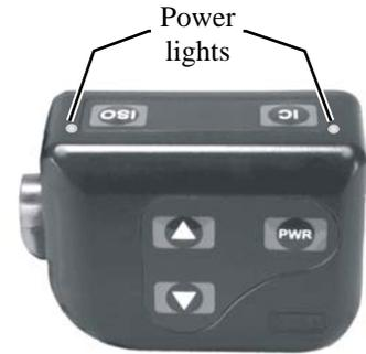
**NOTE:** While the Beltpac is transmitting, the green power light will be flashing.
