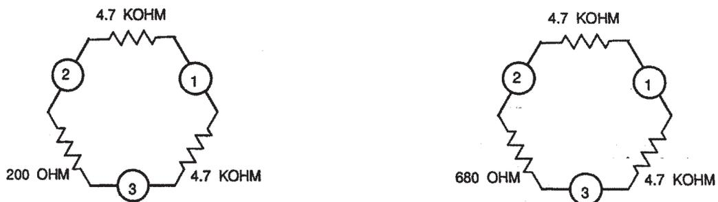
When four-wire outputs are used, termination resistors must be installed for proper operation. The output amplifiers are current sources, and the output level is determined by the terminating
