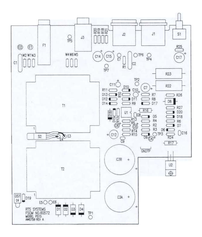
Layout, Printed Circuit Assembly, Model PS15 Power Supply
