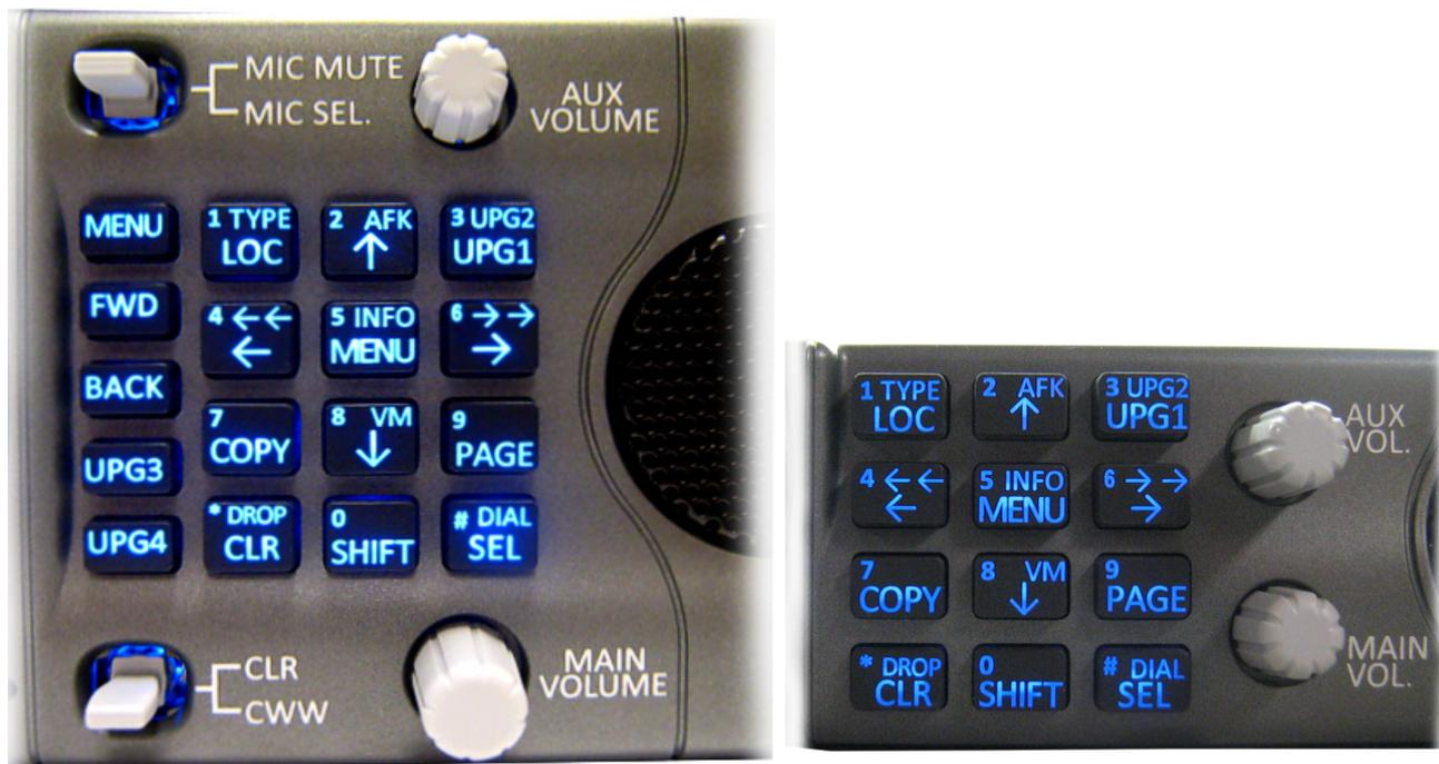
FIGURE 9. KP-5032 Keypad and KP-4016 Keypad
