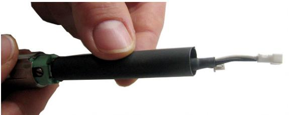
7. Connect the **cable-to-cable connectors**.
