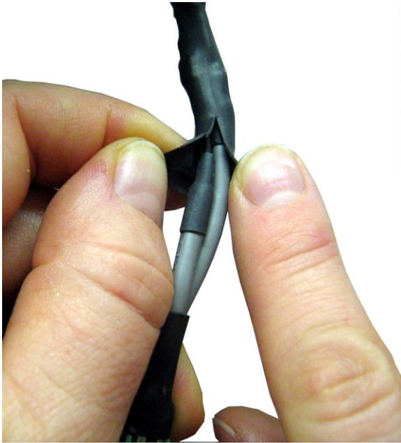
5. Disconnect **both cables** by pulling the cable-to-cable connectors apart.
