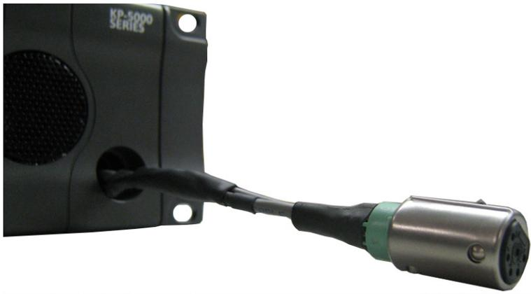
**NOTE:** If the cable assembly becomes caught, shift the cable up and down to clear the cable from the unit.
