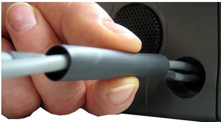
9. Using a heat gun, apply **even heat over the length and diameter of the tubing** (minimum temperature 100°C).
