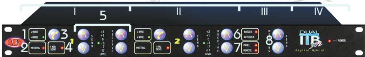
The front panel of AEV ITB-302 is divided into 4 sections.
