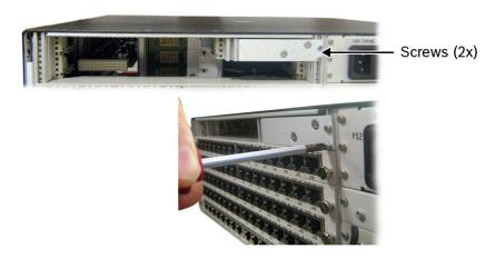
**5.** Using a long shaft Phillips head screwdriver, remove the **collared screw** inside the chassis.
