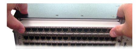
9. Using your fingers or a flat-head screwdriver, tighten the **two (2) thumbscrews** on either end of the backcard into the chassis frame.
