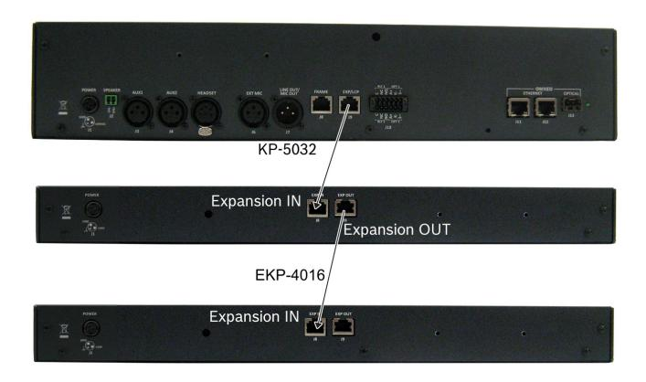
FIGURE 26. Expansion Panel Cabling
