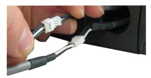
6. Using the replacement headset connector, thread the cables through the supplied shrink-tubing.
