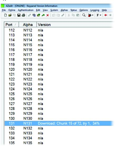
**12.** Verify the keypanel displays the **FPGA Downloading icon with progression bar**. *Once the download is complete, the keypanel has to process the downloaded file.*
