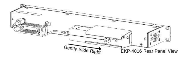
5. Attach the **DC** power connector to the unit.
