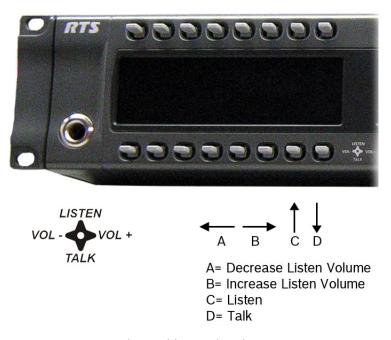
**FIGURE 11.** Key Function Position Explanation
