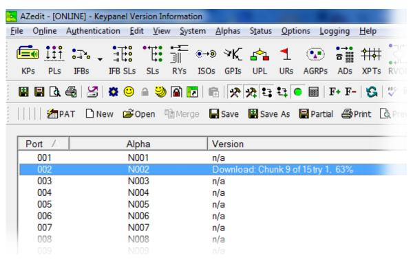
**11.** Verify the keypanel displays the **FONT Downloading icon with progression bar**. *Once the download is complete, the keypanel has to process the downloaded file.*
