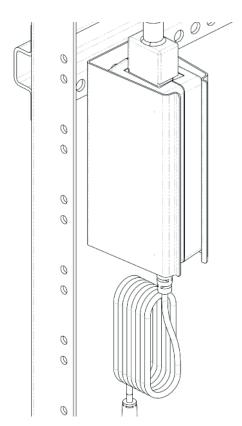
**FIGURE 28.** Mounting Bracket – Vertical from a Crossbar
