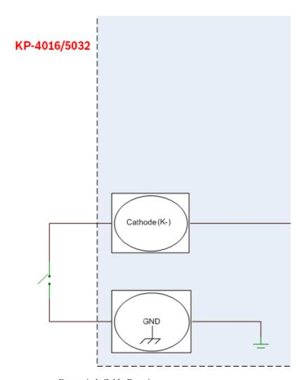
FIGURE 8. Footswitch Cable Drawing
