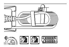
**8.** Attach the **AC power connector** to the power outlet on the power supply.
