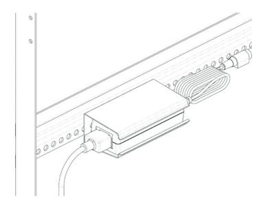
FIGURE 27. Mounting Bracket – Horizontal on a Crossbar
