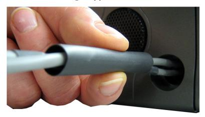
Using a heat gun, apply even heat over the length and diameter of the tubing (minimum temperature 100°C).
