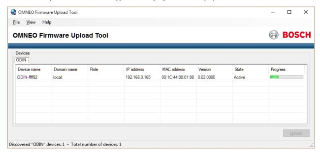
11. Once the firmware has been updated, ODIN reboots and switches into bootloader mode automatically.
