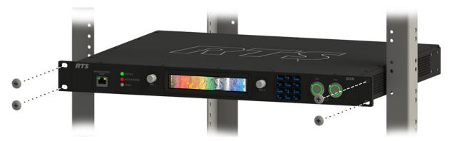
3. On both sides, pass the rear side brackets through the keyhole stand-off (1).
