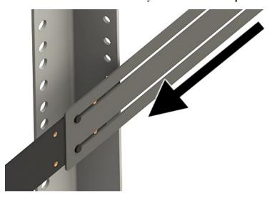
5. Using four rack screws (not supplied), secure the rear side brackets to the rear rack posts.
