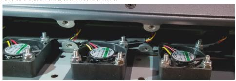
9. Replace the **eight screws**, securing the fan tray to the frame.
