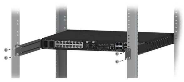
6. Using the supplied pan head screws, internal tooth washers and flat washers, secure the **rear side brackets to the matrix side brackets**.
