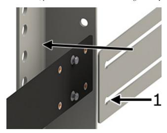
4. Slide the rear side brackets until they reach the rear rack posts.
