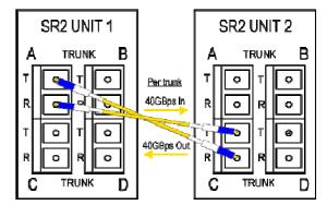
Each trunk is capable of transporting up to 40Gbs of data In and Out. Trunks can be combined to offer more bandwidth or redundancy between network nodes.
